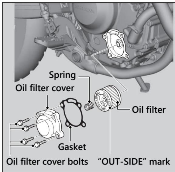
7. Install a new oil filter with the "OUT-SIDE" mark facing out.
