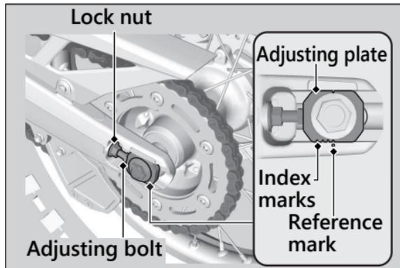
5. Turn both adjusting bolts an equal number of turns until the correct drive chain slack is obtained. Turn the adjusting bolts counterclockwise to tighten the chain. Turn the adjusting bolts clockwise and push the rear wheel forward to provide more slack.
