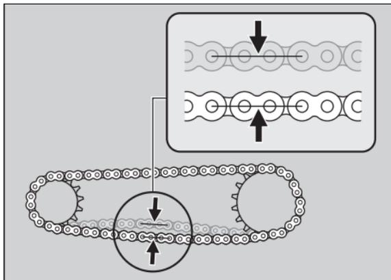
4. Roll the vehicle forward and check that the chain moves smoothly.
